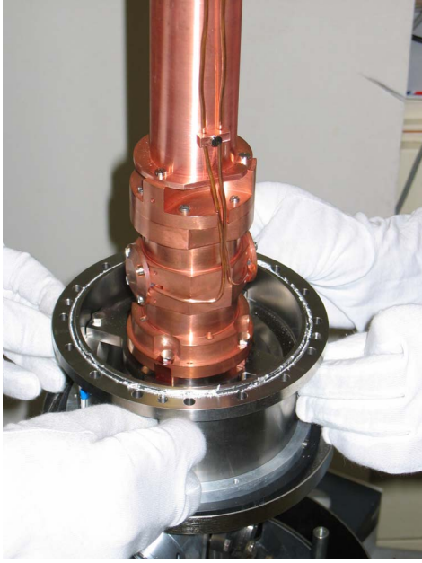
Fig. 1. FOM interrogation cavity with a thermal shield surrounding the drift region above the cavity.
